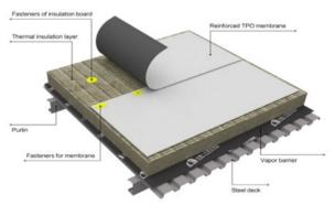
Remark: The figure shows the construction method of the Metal base system.
