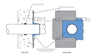
the installation of Bituthene sheet waterproofing membranes. Bituthene Liquid Membrane may be used as a pointing surface sealer for Bituthene sheet membranes. A minimum overlap of the Bituthene sheet membrane of 50mm shall be provided. Bituthene Liquid Membrane is compatible with dry Bituthene Primer, B2 Primer and the Bituthene self-adhesive compound used on all Bituthene systems. Bituthene Liquid Membrane will adhere to clean, dry metal substrates.
